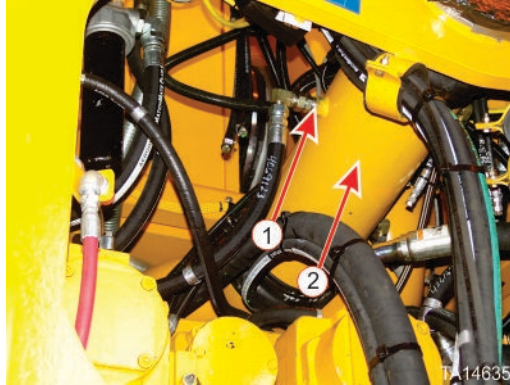
1) Air compressor intake hose connection, 2) Cooling air tube going to front frame
